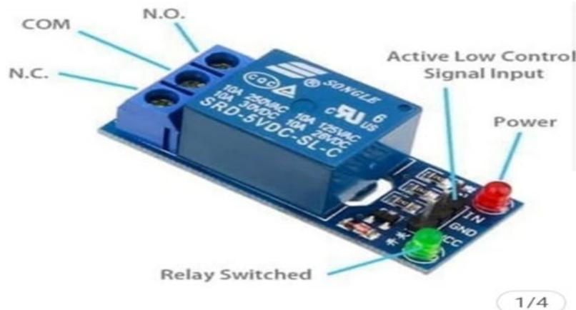
Star Relay Module 1 Channel 10A 250VAC 30VDC Modul DC-AC Low Trigger
